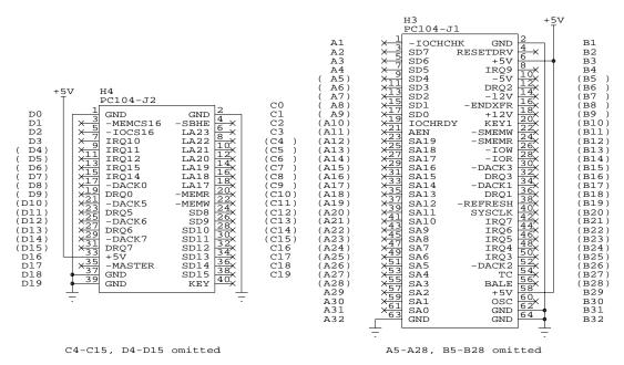
The MB implements a subset of the PC/104 specification in the form of two connectors that provide only +5V and GND for PC/104 modules. Only a total of 32 pins are implemented, 16 on H3 and 16 on H4. By adding up to four 8-pin connectors to the MB, PC/104 modules can be plugged directly into the MB to obtain +5V power and GND. No other connections between the PC/104 bus and the CubeSat Kit Bus are provided.
