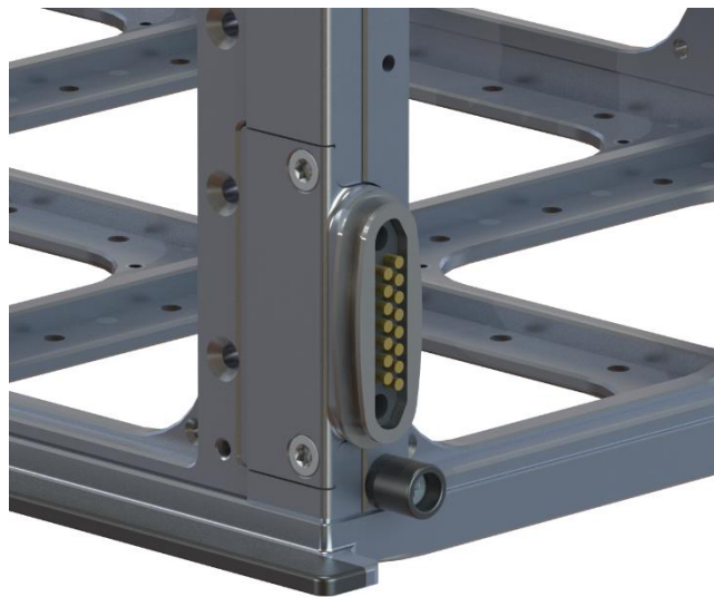
FIGURE 9: PSC SEPARATION CONNECTOR AND PUMPKIN MOUNTING BRACKET
