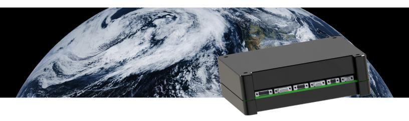
With the NVIDIA Jetson TX2i module at its core, the Zephyr Kestrel adds massive parallel computing capability as well as high-performance CPUs. Zephyr's design adds extra storage, including a standard microSD card and M.2 2280 SSD slot. By default these are populated with validated, industrial-grade options. Gigabit ethernet is available for high-speed connectivity, as well as other common interfaces.
