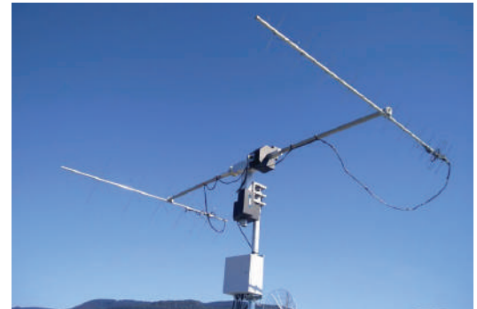
VHF/UHF Ground Station
